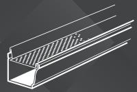
With a continuous hanger™, the rain gutters are reinforced along their entire length.
